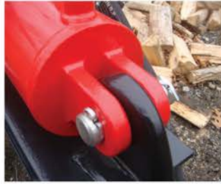
Heavy duty welded 5" cylinder with 24" stroke
