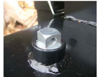
Eight gallon tank with pre-filter & vented cap with dipstick
