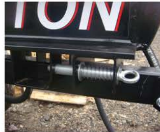
Self-locking pin holds beam in horizontal position
