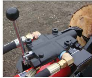
Single spool valve with auto-kick-off detent
