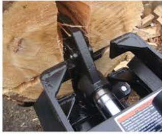
Optional 4-way wedge doubles efficiency
